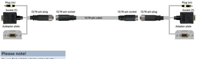
You can find suitable adapter plates for the 13/19-pin installation cable on page 104 - 105
