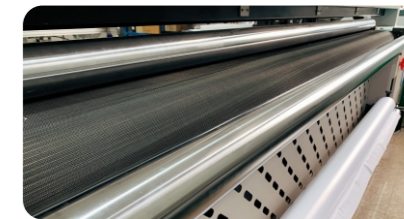
Strengthful chrome plated shaft, to secure the feeding of media straight and flat, for better print output.
