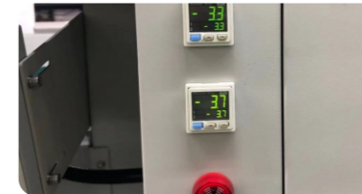
Individually controlled negative pressure system for stable ink supply.
