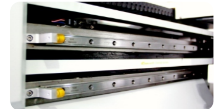
Double silent guide, for speedy and stable carriage moving.
